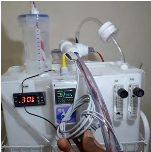
Figure 6: PoliteheartCPAP with incorporated pulseoximeter (P)
